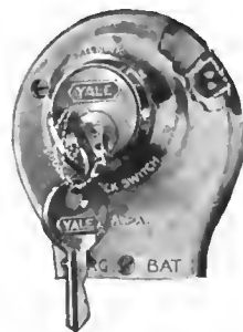
Goodrich switch lock. By its use the switch is locked when the motor is shut off
